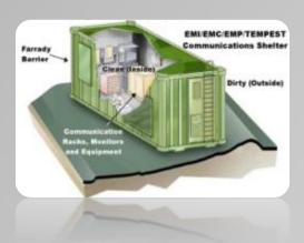
reduce the coupling of EMP electric and magnetic fields into the protected area. The electromagnetic barrier shall consist of the Facility HEMP Shield and protective devices for all POE's. Additionally, reliability, maintainability, safety and human engineering, testability, configuration management and corrosion control all need to be incorporated to the HEMP protection system design.
