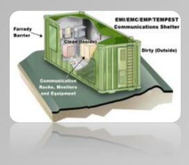
reduce the coupling of EMP electric and magnetic fields into the protected area. The electromagnetic barrier shall consist of the Facility HEMP Shield and protective devices for all POE's. Additionally, reliability, maintainability, safety and human engineering, testability, configuration management and corrosion control all need to be incorporated to the HEMP protection system design.
